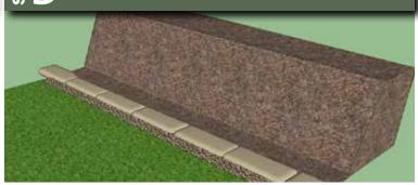
Fill the space behind the bags with backfill material and rake level so that the material is slightly higher than the bags.
