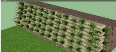
Repeat steps 3-6 until you reach your desired bed height. Be sure to set the bags in a brick pattern, so that the bag above spans the seam between two bags below by at least 8". Backfill behind each course once completed. Level bags as needed by adjusting the snorkel wrap length.
